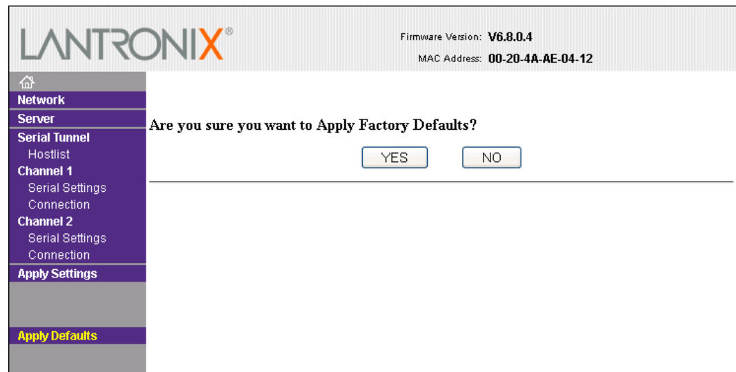
Figure 5-10. Applying Default Settings
